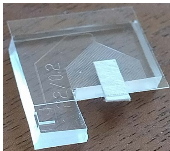
figure 1: shows the mechanically integrated paper and PDMS microfluidic system
