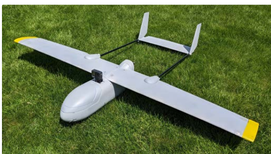
Second prototype UAV with autonomous flight capabilities and IoT telemetry link
