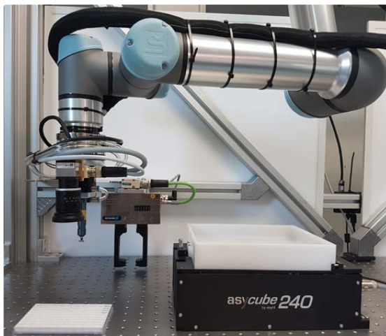
Figure 1: UR5e robot performs an example task. The links are placed in a pallet, which can be exchanged automatically.
