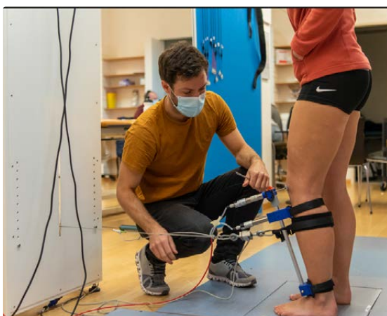
Fig 1: Current prototype tested in a static measurement to simulate an external shock force with an apposite apparatus
