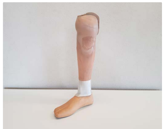
3D printed ankle cover mounted on the prosthesis supplied by Botta Orthopädie AG.
