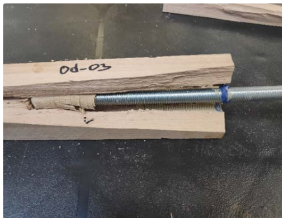
Figure 1: Timber splitting failure
