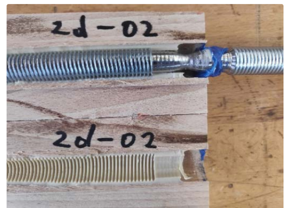
Figure 2: Ductile steel failure
