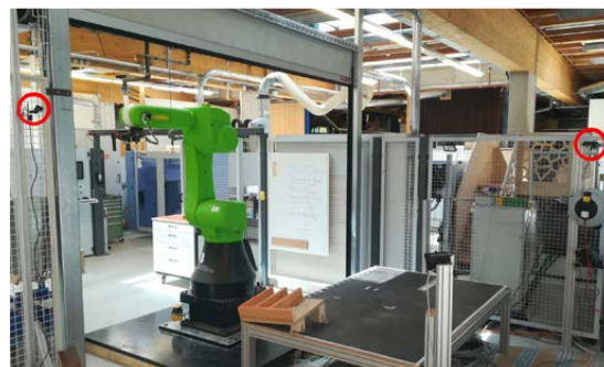
Figure 2: Fanuc CR35-i robot and its workspace, including both Asus Xtion Pro cameras (marked with a circle).
