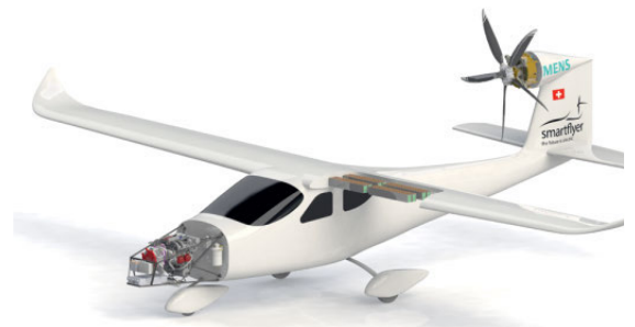
Batteries, combustion engine and electric motor placed inside the airplane.
