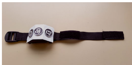
Concept of attachment to the human body and structural solution for the detection of the rotation direction.
