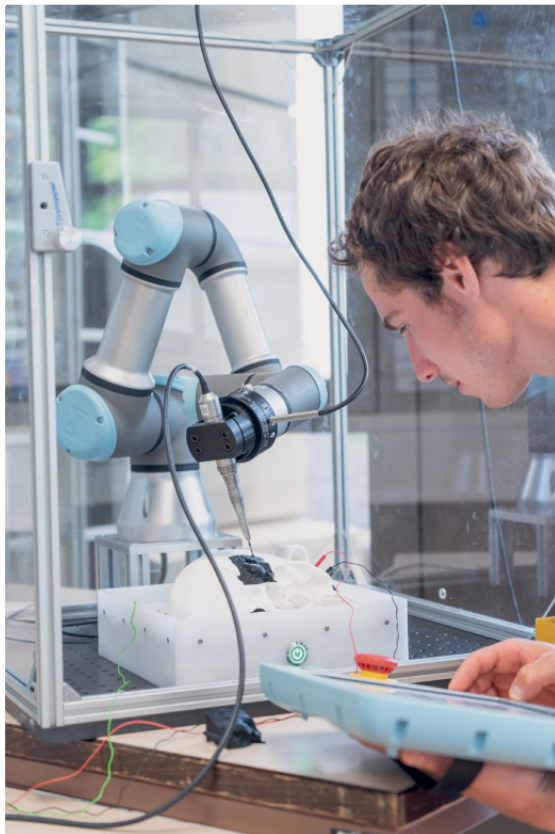
The test arrangement shows the programmed robot guiding the prototype drill into the head-phantom
