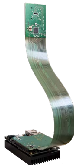
Figure 1: Semi-Flex PCB with the CCD line sensor
