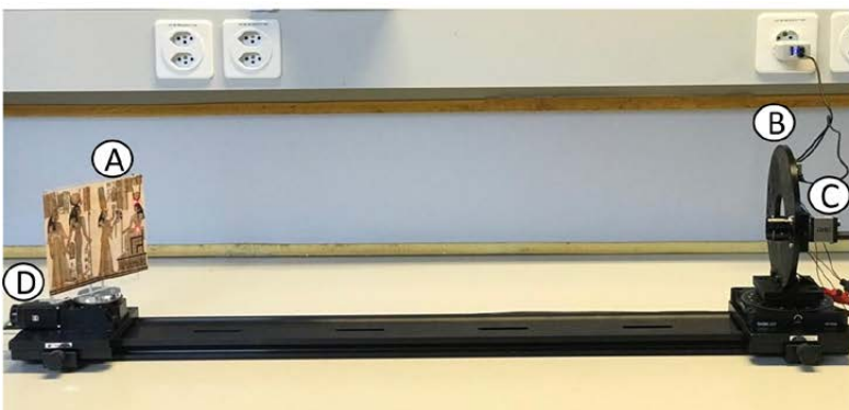
A)Historical image, B)Prototype of the system, C)Small camera, and D)Stepper motor to rotate the image
